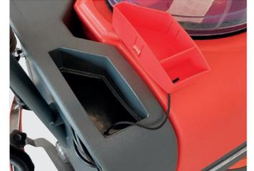
Filling hole for fresh water tank
