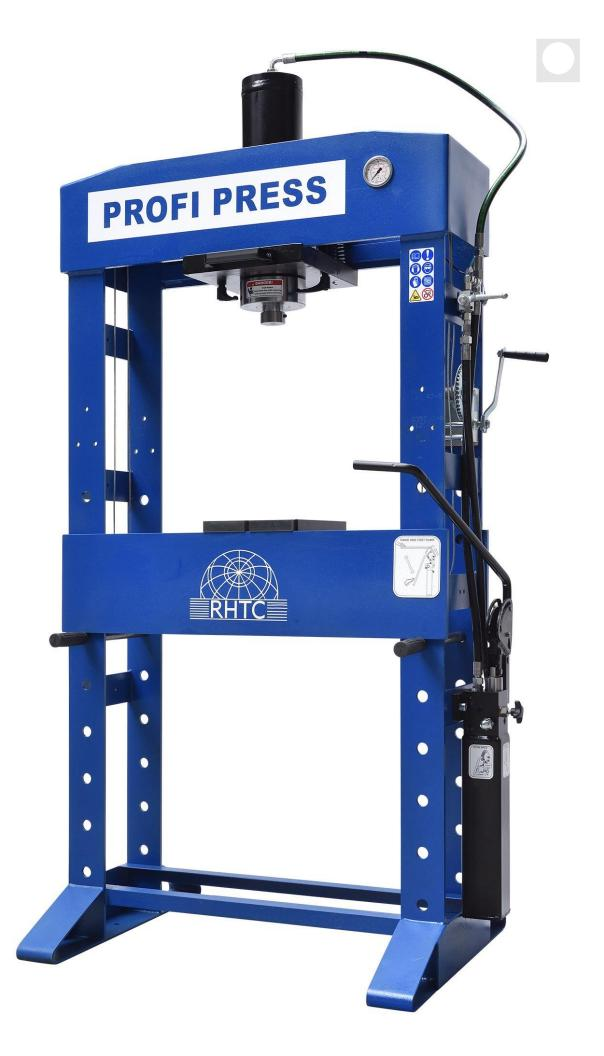
Our manual hydraulic press (50 ton HF-2) can be operated by hand as well as by foot: the handpump is interchangeable to a foot pump. This workshop press has a movable cylinder and the height of the work table is easy to adjust with a winch. Thanks to the inheight adjustable work table of this hydraulic press, you can easily work with di erent material / product sizes.
